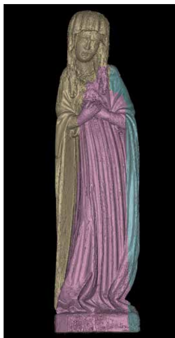
17 Our Lady of Sorrows from Krupka, examination with the use of computer tomography – 3D modelling with the individual wooden blocks indicated through different colours. Photo: Jakub Pečený.
